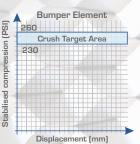
A complete testing procedure for certification of aluminum honeycomb is performed in-house according to the NHTSA Lab Test Procedure for Dynamic Side Impact Protection: TP214D Appendix C. The side impact barrier materials having crush strength of 45 PSI +/- 2.5 PSI for the main block and 245 PSI + 15 PSI for the bumper block.
